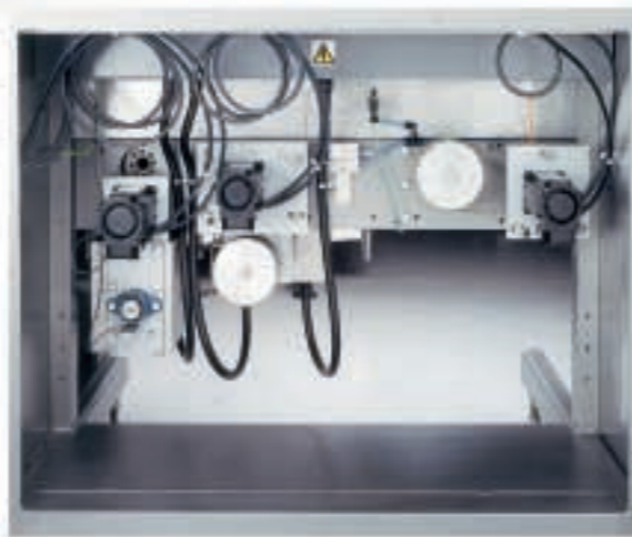
Interior of a Flowtronic 120 showing individual servo motors on each axis
